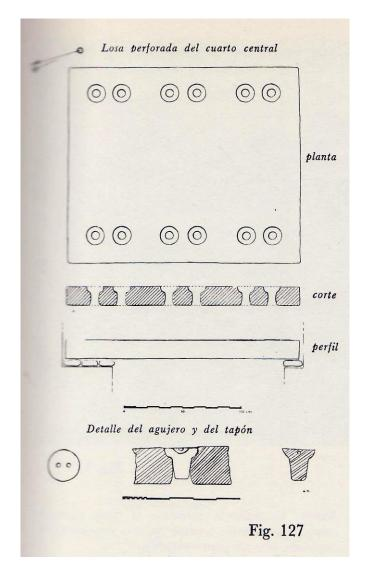
**Figure 6.5** Drawing Displaying the Arrangement of Holes in the Cover to the Temple of the Inscriptions Stairway (Source: Ruz 1973:124)
